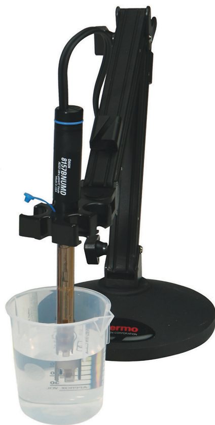
Figure 2. Electrode in cleaning solution
