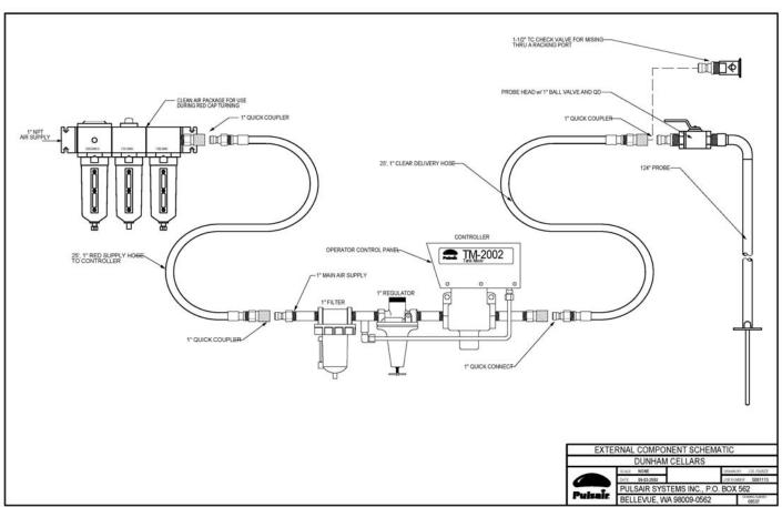
The external component schematic shows the connections and layout of a TM-2002 System. The clean air package on the left is connected to the compressed air source. The TM system is packaged with both a supply and delivery hose that are 25 feet in length. The output from the TM can be connect to the probe or to the
