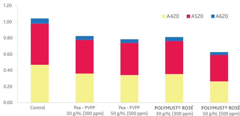
*Static fining trial at 7°C (44.6°F) before AF, Modified Colour Intensity measures.
