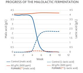
Experimental result demonstrating the ability of fumaric acid to block malolactic fermentation. L-lactic acid is still not detected 10 weeks after treatment while MLF is completed in the control.
