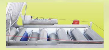
All parts that come into contact with the product are foodcontact compliant. All parts are made from stainless steel to fully meet the strictest hygiene requirements for food and drink processing.
