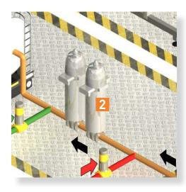
Pre-stabilization refers to the fine filtration of bright beer, beer which has already been clarified, to reduce the level of microorganisms and turbidity prior to further downstream processing / storage.
