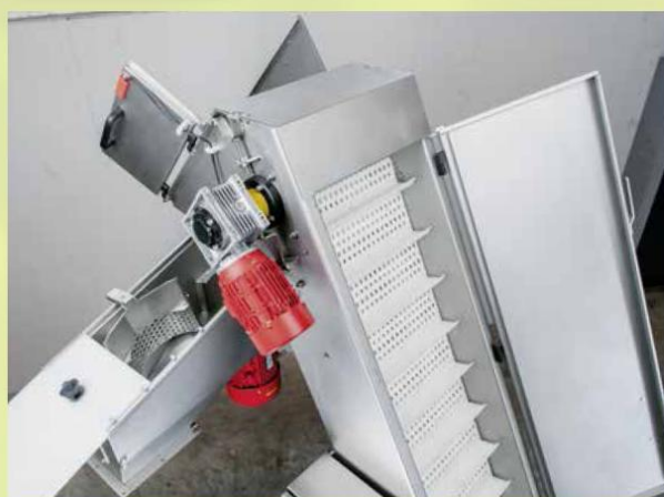
The diagram shows the SA400-RM40 with open doors and centrifugal mill removed
