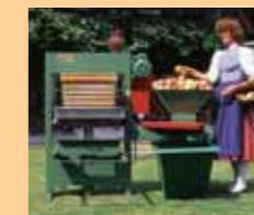
The optimum pressing system for best quality juice (aroma, fresh flavour, cloudy content) and top yield due to a multiple sub-divided press head giving the juice an immediate free flow with resultant high working speed.
